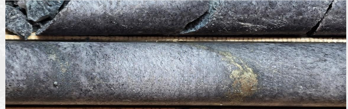
Figure 2: Example of minor Cu mineralization in PN-24-090 drill core that led to BH EM discovery in PN-24-094
